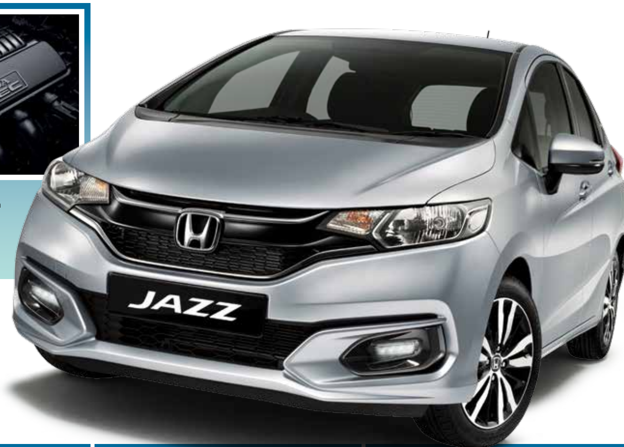
1.5L i-VTEC Engine Inject fun into every drive so you can travel more miles with a smile. Maximum power: 120PS [88kW] / 6,600rpm Maximum torque: 145Nm [14.8kg-m] / 4,600rpm
